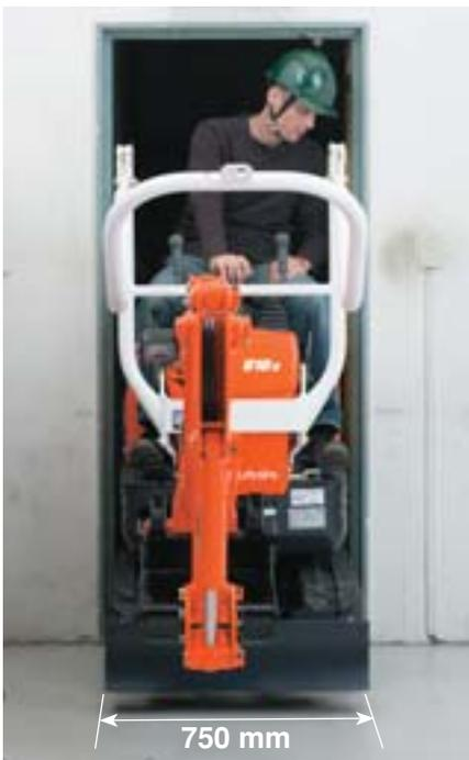
When adjusted down to 750 mm, the U10-3 can easily fit through most doorways, permitting access inside of buildings.
